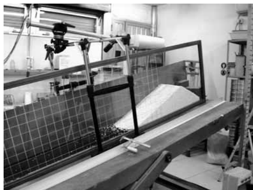
Fig. 1 - Laboratory flume and laser-scanner apparatus testing low density PVC material
