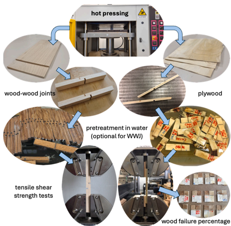
Fig. 3. Sequence of sample preparation and mechanical testing.
