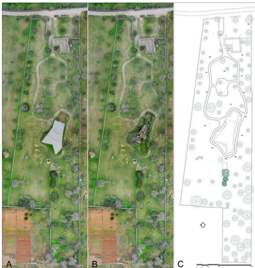
Figure 4. The 3D survey: (A), the digital aerial photogrammetry of the archaeological site; (B), the aerial survey merged with the digital close range photogrammetry of the tombs current visible under the metal cover; (C), CAD plan.
