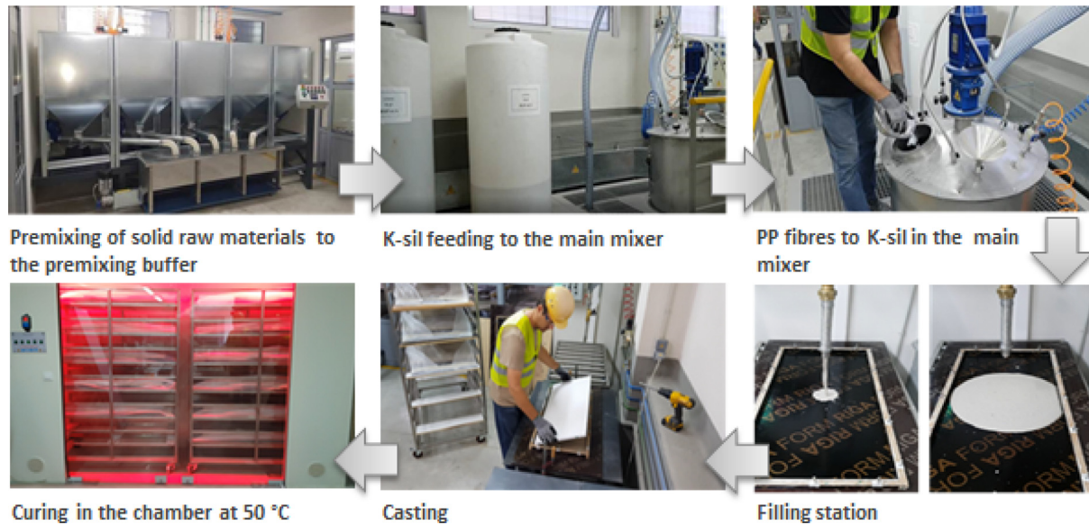
Fig. 2. The “modular” production line.
