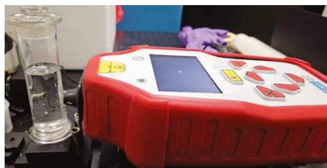
Figure 1. Photo of the hand-held SORS instrument and historic glass jar containing preservation fluid.
