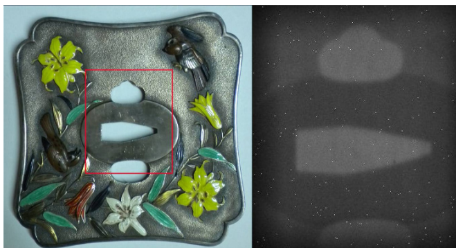
Fig. 4: (Color online) Left: picture of the tsuba (6 cm \times 6 cm size and 4 mm nominal thickness). Right: neutron radiography of the irradiated area marked by the red square in the picture on the left.
