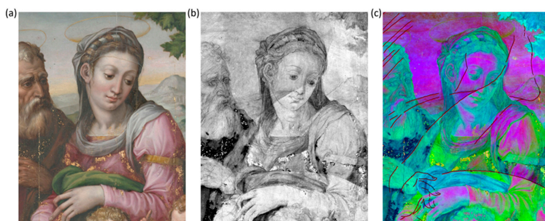
Figure 3. Detail of the visible depiction in the RGB image (a) and of its underdrawing in the NIR at 1830 nm (b); PC color-composite image (c) obtained by combining PC1, 2, and 3 (inverted).
