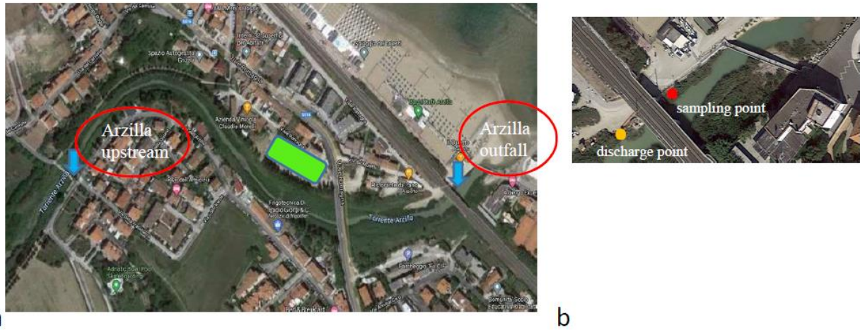
Figure 6.3 - 1 Study site and sampling strategy; a) two sampling stations are positioned along the Arzilla River, Arzilla outfall (where is located the automatic water sampling for microbiological and chemical analyses) and at Arzilla upstream; b) discharge point or CSO (combined sewer outflow) and automatic sampling station.
