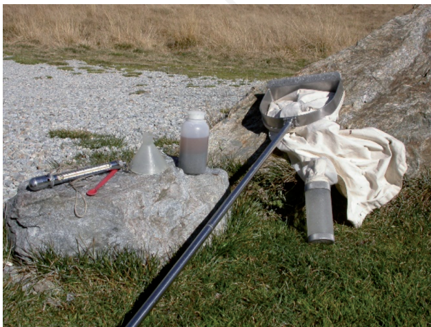
Fig. 3. Handled net, field thermometer, bottle and funnel useful for collecting and treating macro-fauna samples in the field (left). Surber net for collecting meio-fauna samples and filtering procedure (right).
