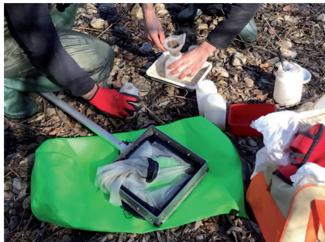
Fig. 3. Handled net, field thermometer, bottle and funnel useful for collecting and treating macro-fauna samples in the field (left). Surber net for collecting meio-fauna samples and filtering procedure (right).
