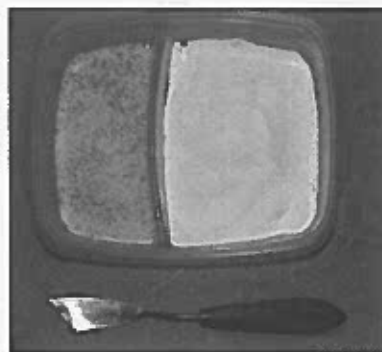
Figure 4. The raw materials used to reproduce the ancient mortar: on the left the aggregate and on the right the powder of MgO.
