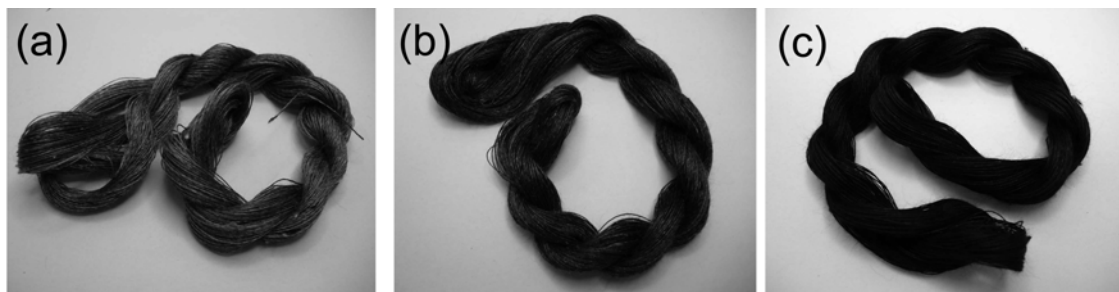
Figure 8. Pictures of spun silk yarns with (a) 30 w%, (b) 60 w%, and (c) 100 w% PPy-coated silk fibers.
