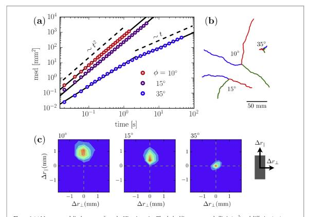
**Figure 6.** (a) Mean squared displacements from the 2D trajectories. The dashed lines represent ballistic ( $\sim t^2$ ) and diffusive ( $\sim t$ ) behaviour. (b) Sample trajectories for structures with varying leg tilt angle. (c) Probability distributions of parallel and orthogonal displacements (Dt = 40 ms) with respect to the orientation of the structure.
