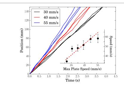
Figure 5. (Main panel) Displacement of the walker (on a single lane track) as a function of time for different values of the maximum plate speed. The object has thin (flexible) legs with tilt angle f=15 [IIII] Inset) Average speed of the walker versus the maximum plate speed (points), the line is a linear fit passing through zero.
