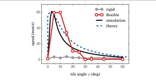
**Figure 2.** Average speed as a function of the leg tilt angle in experiments, theory and simulations. A clear peak at around f » 10 is found for flexible structures.
