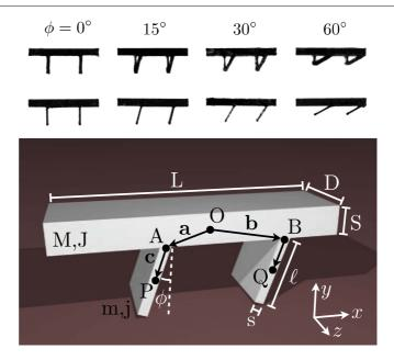
**Figure 1.** (Top panel) Photo of the 3D printed walkers used in the experiment, structures in top row have connected (rigid) legs and structures in bottom row have free (flexible) legs. (Bottom panel) Scheme of the idealized walker considered in the theory.
