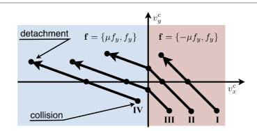
Figure 3. Collision types: (I) the horizontal contact point speed  $v_x^c$  is positive throughout the collision, (II)  $v_x^c$  is positive at maximum compression  $v_y^c = 0$  but becomes negative during restitution, (III)  $v_x^c$  becomes negative before maximum compression, (IV)  $v_x^c$  is always negative.
