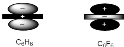
Figure 31. Representation of the quadrupole moments of benzene and hexafluorobenzene. Adapted with permission from ref. 439. Copyright 2002 John Wiley and Sons.
