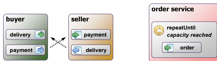
Figure 1: Services with incompatible behavior (the buyer and seller services wait for each other) and an ill-designed service (a partner of the order service would have to guess the service's capacity).
