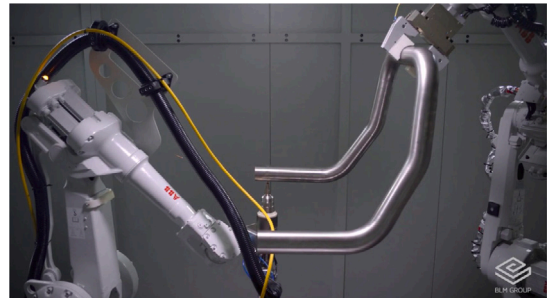
Fig. 1. Laser Cutting performed by two cooperative Robot (LT360 from BLM Group, [1]).
