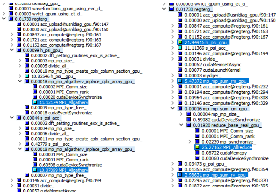
Fig. 12. Profiling summaries visualised from CUBE and obtained with Score-P by instrumenting the CPU only at 96 GPUs (24 nodes, nb = 4 ). The panel on the left shows the percentage of time spent in MPI_Allgatherv from the different calling paths; the same information is provided for MPI_Allreduce in the right panel.
