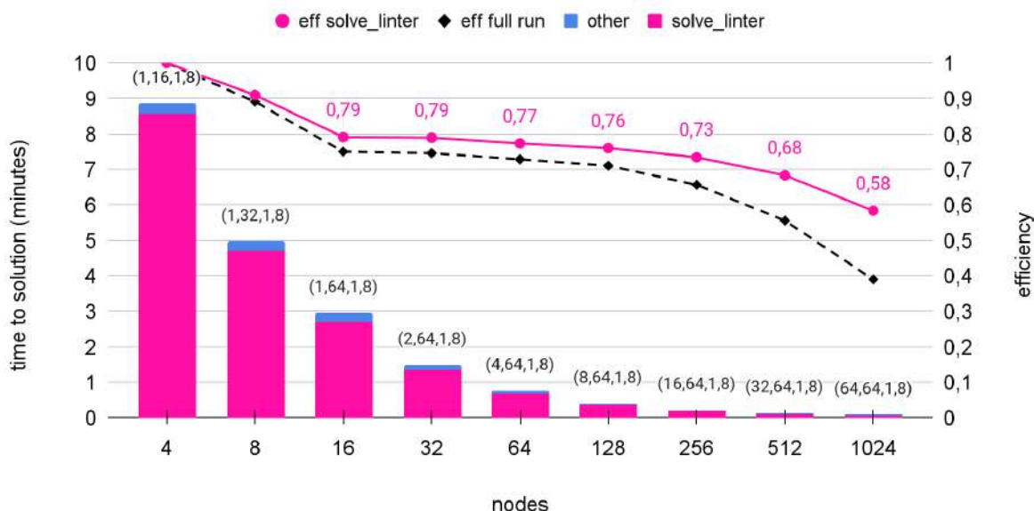
Fig. 6. Walltime of the PHONON runs on Leonardo (columns). Most of the time is spent in the solve_linter kernel (purple section) to compute the contributions to the dynamical matrix by an irreducible representation. The system is scaled on pools up to 64 GPUs, which is the largest number of pool processes available for this workload; further scaling is achieved up to 64 images. We could in principle reach 192 images, but we could not further scale the application due to the limited availability on Leonardo's booster partition at the time of the benchmark. The numbers between brackets on top of the columns represent the parallelization adopted, according to the notation (n_i, n_k, n_{pw}, omp) , where n_i is the number of images, n_k the number of pools, n_{pw} the number of R&G processes and omp the number of openmp threads. The black dashed line is the efficiency of the whole simulation, while the purple continuous line refers to the efficiency of solve_linter routine.
