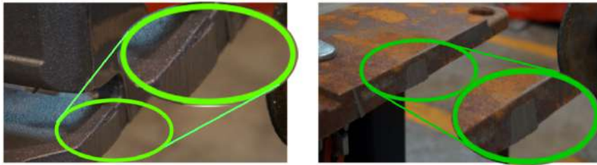
Figure 3. Burrs are not completely removed due to the deflection of the mechanical structure of the spindle.
