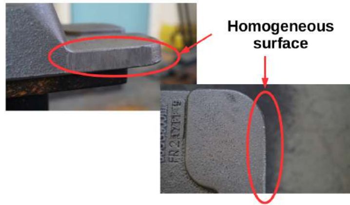
Figure 14. T2 experiment results: workpiece surface after burr removal exploiting the human mimicking control strategy.
