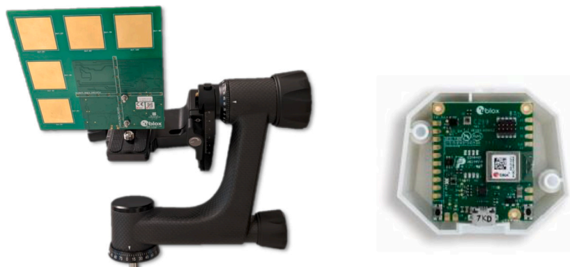
Fig. 11. Ublox anchor mounted on a graduated gimbal and tag.
