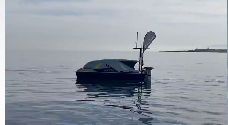
Crete cal&val campaign: ASV equipped with multibeam sonar, pH sensor and passive acoustic sensor
