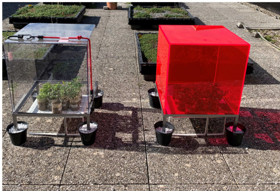
Figure 5. Picture of outdoor experiments. The boxes are made of transparent polycarbonate and red LSC panels. Note: pots filled with white stones at the base of the box structures have the only function of anchoring the panels to avoid possible adverse effects in the event of a mighty wind.
