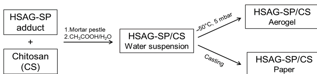
Figure 2. Block diagram describing the preparation of high surface area graphite with serinol pyrrole and chitosan (HSAG–SP/CS) water suspensions, aerogels and papers.
