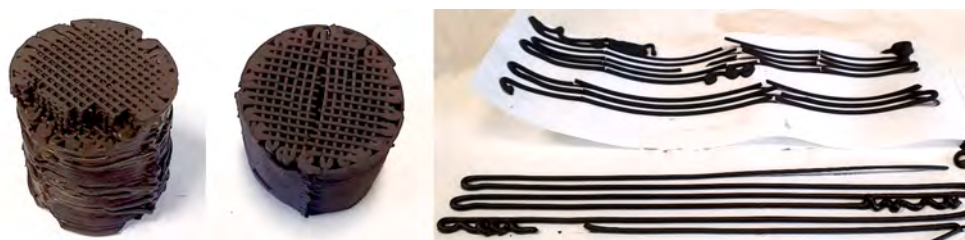
Fig. 4. Failure in printing CZA:H-ZSM-5 catalysts at an early stage.
