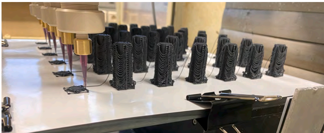
Fig. 9. Scaling up of CZA-based 3D printed catalysts.
