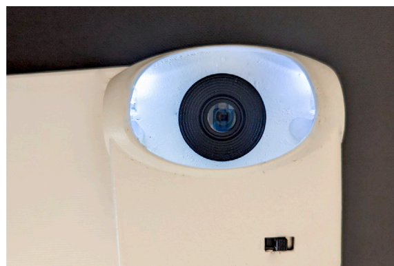
Fig. 1. Close-up view of the spacer on our device, with the LED turned on.
