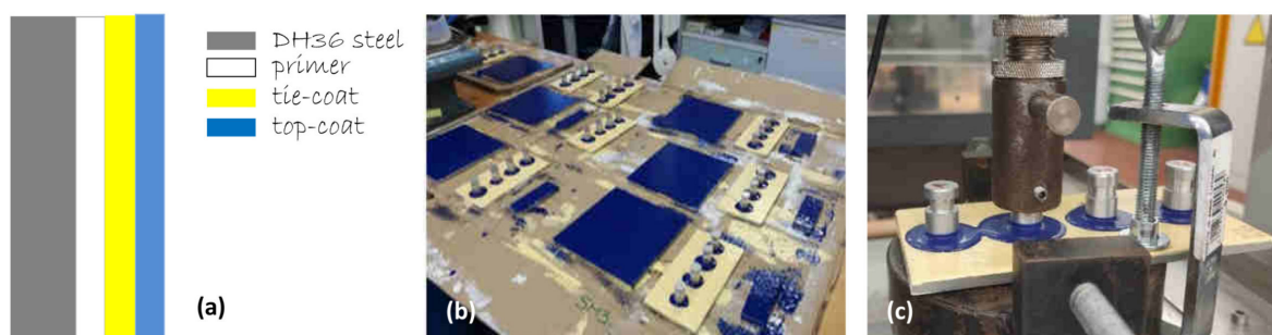
Figure 1. Scheme of layers deposited on the DH36 steel (a); image of the painted steel samples for the mechanical adhesion tests (b); image of the experimental set-up for the pull-off test (c).
