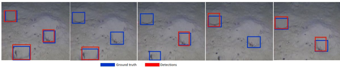
Figure 4.1.1: Ground truth (blue color, bounding boxes). The result of detector (Inception) (red color, bounding boxes). Due to camera angle variation and burrows appearance, the detector missed detections in consecutive frames.
