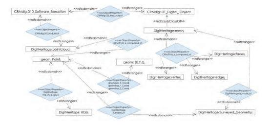
Figure 3 Ontology representation for Phase 2 – Point clouds to meshes or geometries
