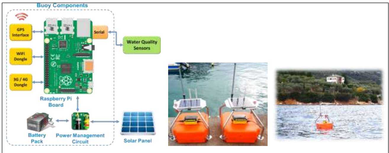
Figure 6. NITOS Buoy node architecture, nodes before deployment and buoy nodes deployed.
