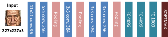
Fig.3. Architecture of AlexNet. It consists of five convolutional layers, some of which are followed by maximum pooling layers and then three fully-connected layers and finally a 1000-way softmax classifier.
