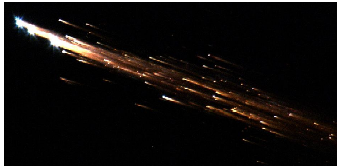
Figure 6 - The controlled re-entry and subsequent breakup and fragmentation of the European Space Agency's "Jules Verne" Automated Transfer Vehicle (ATV) 30 .
