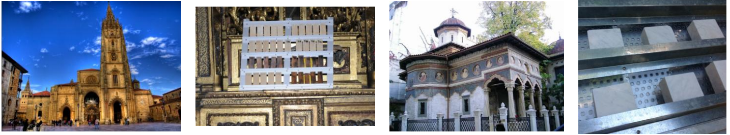
Figure 1. Examples of field tests on wood and stone specimens running at Oviedo Cathedral and Stavropoleos Monastery (Bucharest) respectively.
