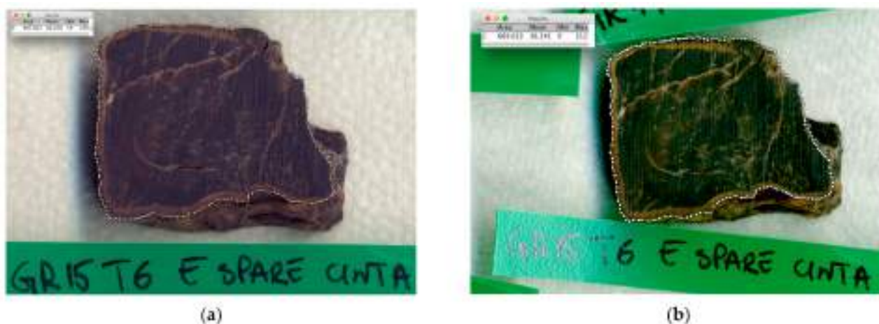
Figure 2. An example of how the surface area changes were calculated using the ImageJ software: (a) the initial area of sample T6 E; (b) the same area after conditioning in the climate at 35% RH.
