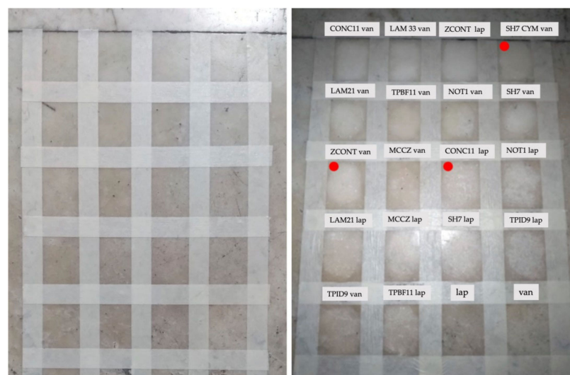
Figure 9. Result of preliminary tests on site before and after the removal of micro-packs containing different bacteria. The red dot indicates the bacterial strains chosen by the quality of the cleaning.
