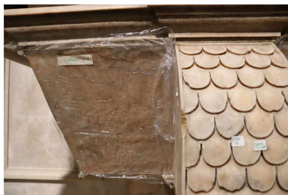
Figure 5. Lateral left side of the sarcophagus covered with micro-pack with different bacteria.
