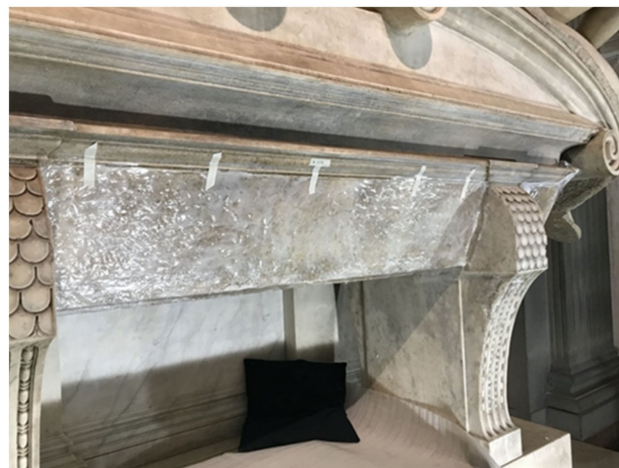
Figure 4. Front side of the sarcophagus covered with a micro-pack of S. ficaria SH7 in vanzan.
