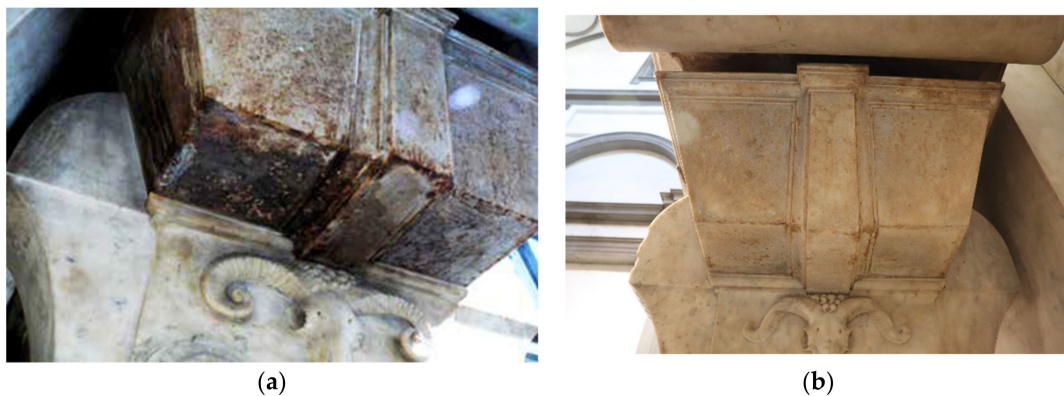
Figure 10. Right side of the sarcophagus, before (a) and after (b) the bio-cleaning treatment.
