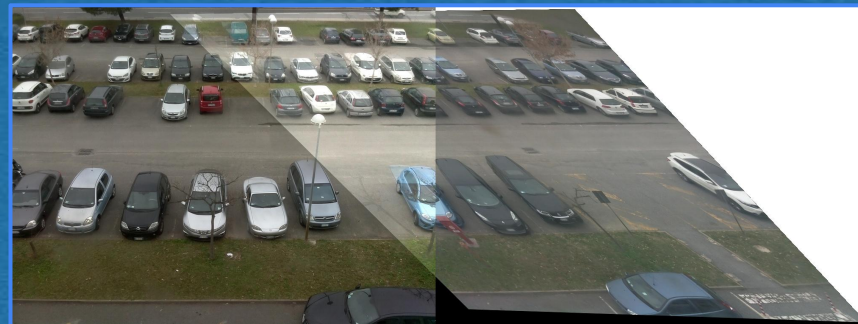
Stitching of two images coming from two neighboring cameras. We exploited the computed homography matrix.
