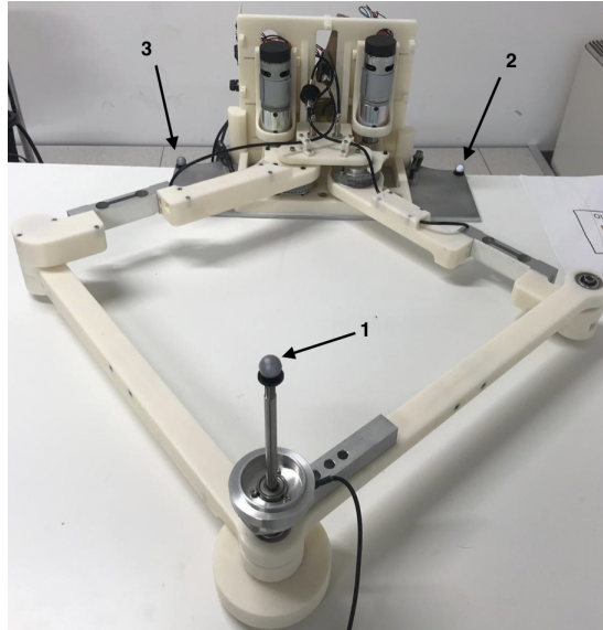
Figure 20. Placement of the markers on the prototype for the experimental procedure.
