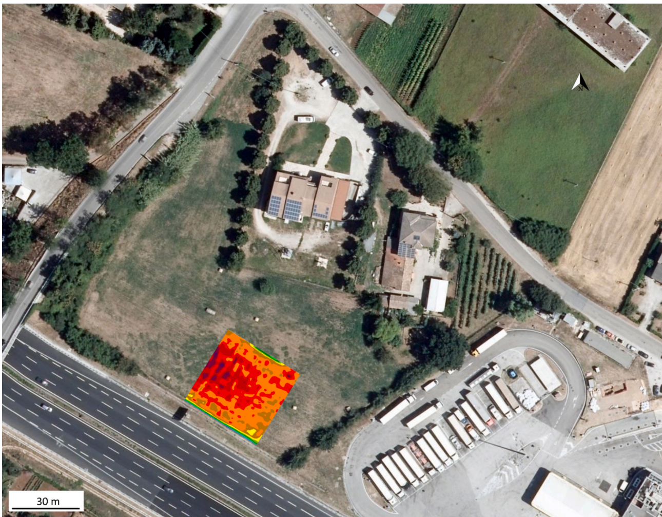
Fig. 13. Georeferenced map of resistivity at depth range 0.35–0.75 m.
