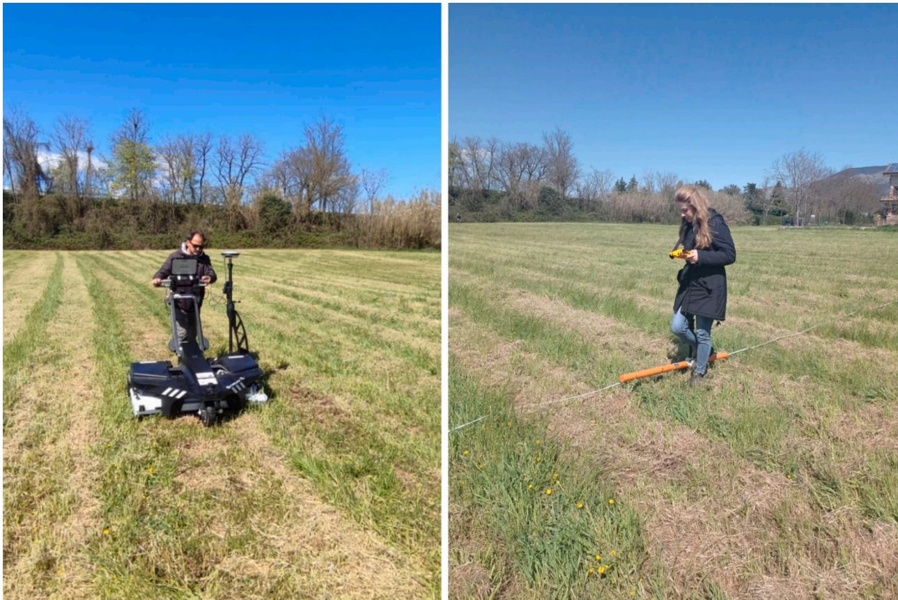
Fig. 4. Geophysical instruments: Stream C multichannel GPR on the left; electromagnetometer mini explorer on the right.
