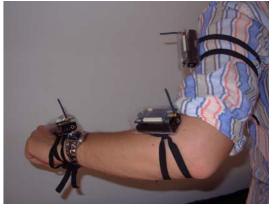
Figure 4. A detail of the body area sensor network.
