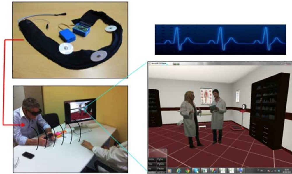
Figure 7. Setup of the VR system used in the clinical setting. Top left: personal bio-monitoring system. Bottom right: example of a stressful scenario used in the training.
