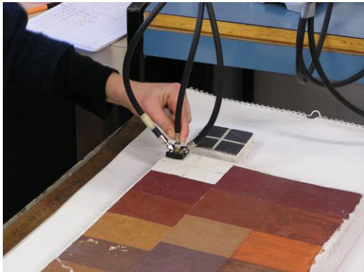
Fig. 3: FORS measurements on mock-up.
