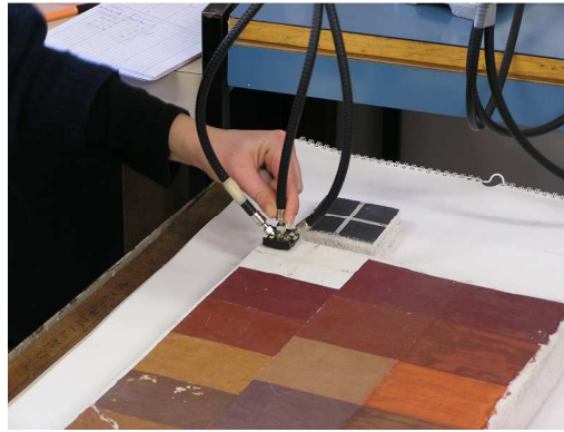
Fig. 3: FORS measurements on mock-up.
