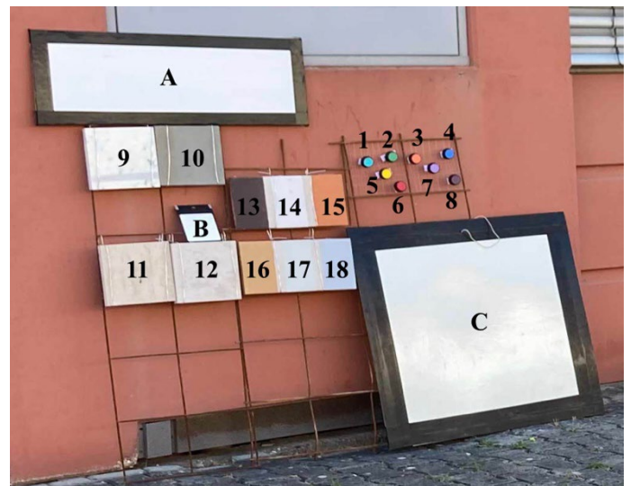
Fig. 3 – Mockups, stones and Spectralon® Color Standards arranged in the grid.
