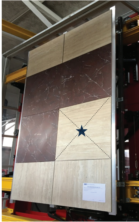
Figure 22. Position of the accelerometer on the tested specimen.
