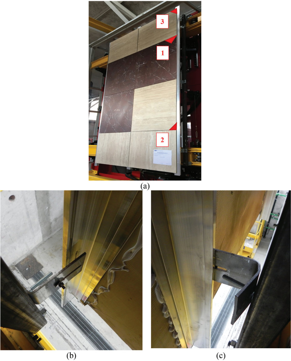
Figure 24. Damages occurred during the in-plane crescendo test: (a) detachment of portion of porcelain tiles; (b) brackets bolt leaving the guide and (c) yielding of the bottom brackets.
