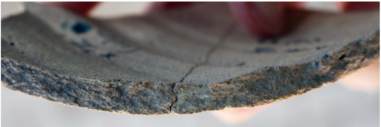
Figure 3: Irregular profiles and discontinuities in cross-sections typical of the geometric painted specimens.
