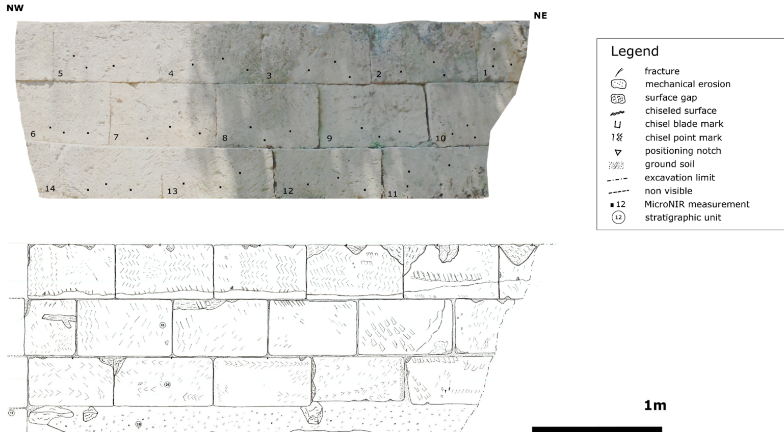
Figure 6. Documentation of one portion of the fortification wall at the site of Porta Schiavone, Montescaglioso [24].
