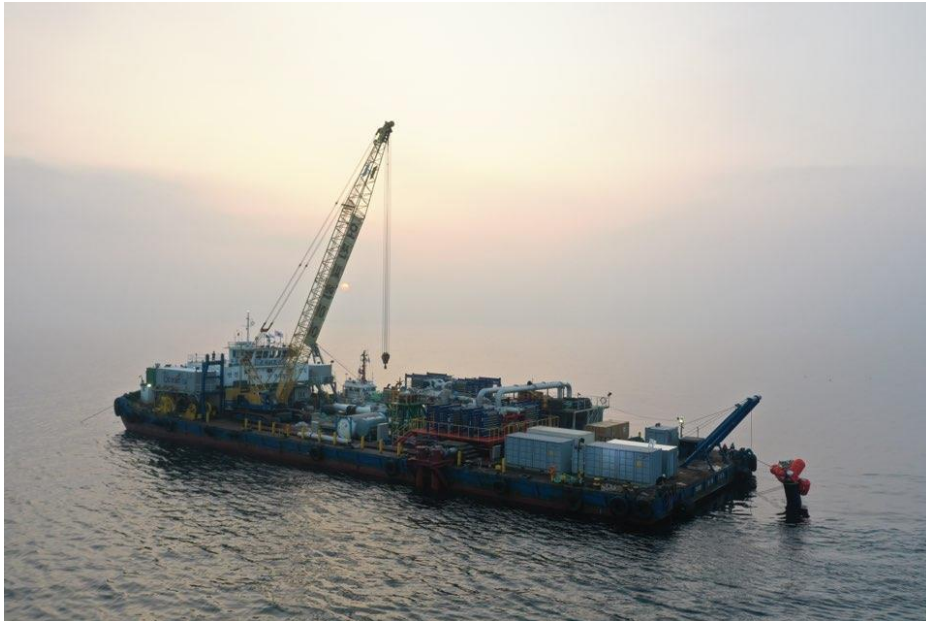
Figure 1: The 1-MW OTEC plant on the barge with the riser (Seo and Kim, 2019).
